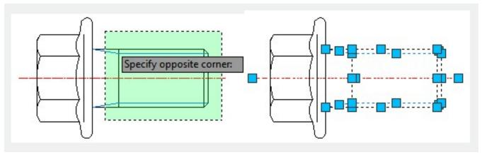
When you use window selection, if an object with a dashed linetype only partially visible in the viewport and all visible vectors of the linetype can be enclosed within the selection window, the object can be selected.
