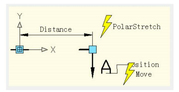
Pick the right grip of the Polar Parameter as an associated parameter point and specify the Stretch box as below:
