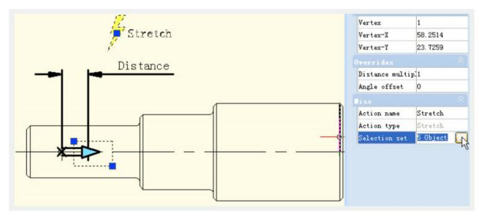
The black object is the operational object of the action, the broken line frame is the stretch frame, objects intersect with stretch frame will be stretched, objects which will be selected by the stretch frame will move.
