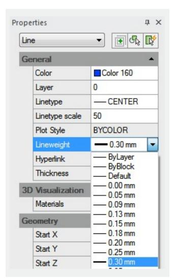
Usually the objects are created with the lineweight assigned to the current layer. If the current lineweight is set to BYBLOCK, objects are created with the default lineweight setting until the objects are grouped into a block. If you do not want to use the lineweight currently assigned to the layer, you can select any other lineweight for object.
