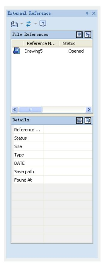
The Xref Manager dialog box is used to edit and control external reference in current drawing.
