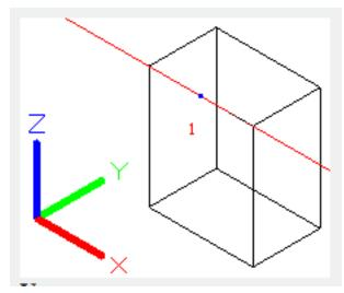
**Ver :** Create a vertical xline through specified point. This xline is parallel to Y axis.
