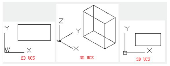
**3D:** if the current UCS is the same as WCS, looking down the UCS (the positive direction of Z axis), the origin in XY plane displays as a box; looking up the UCS, the box disappears.
