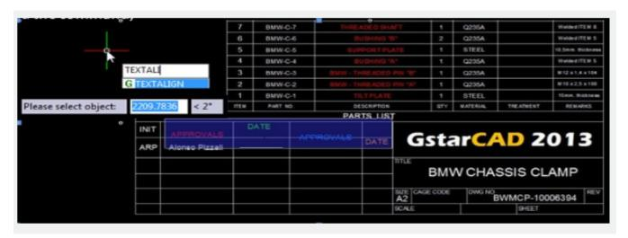
After selecting the text(s), a message will display > Select the align method: X axis (X) / Y axis (Y) / Two points (P):
