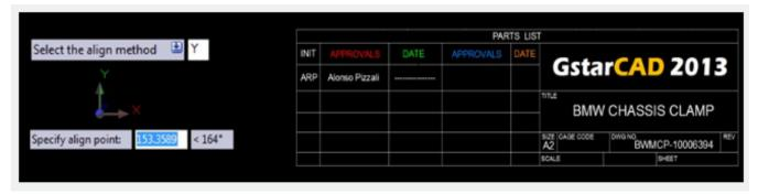
In another example, we choose the X axis alignment method and then specify a point to align the texts in the correct location (end point of Leader). The result is as follows:
