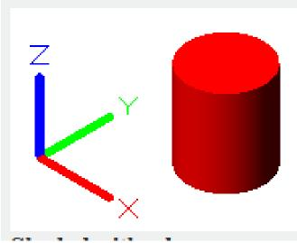
**Shaded with edges:** Create smoothly shaded models with visible edges
