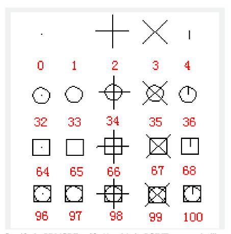
Specify the PDMODE to 32, 64 or 96; the POINT command will not only draw graph of the point, but also display graph around the point.
