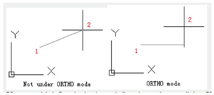
Users could define the horizontal direction to be parallel to X axis of UCS and the vertical direction to be parallel to Y axis of UCS. In 3D viewport, the ORTHO is defined to be parallel to Z axis of UCS. The command prompt displays +Z or -Z according to angle of Z axis.
