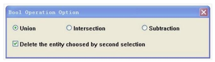
Delete the entity chosen by second selection: Choose whether to delete the second selected object. There are different Boolean operation options such as union, intersection and subtraction. After the operation the object will be a polyline.
