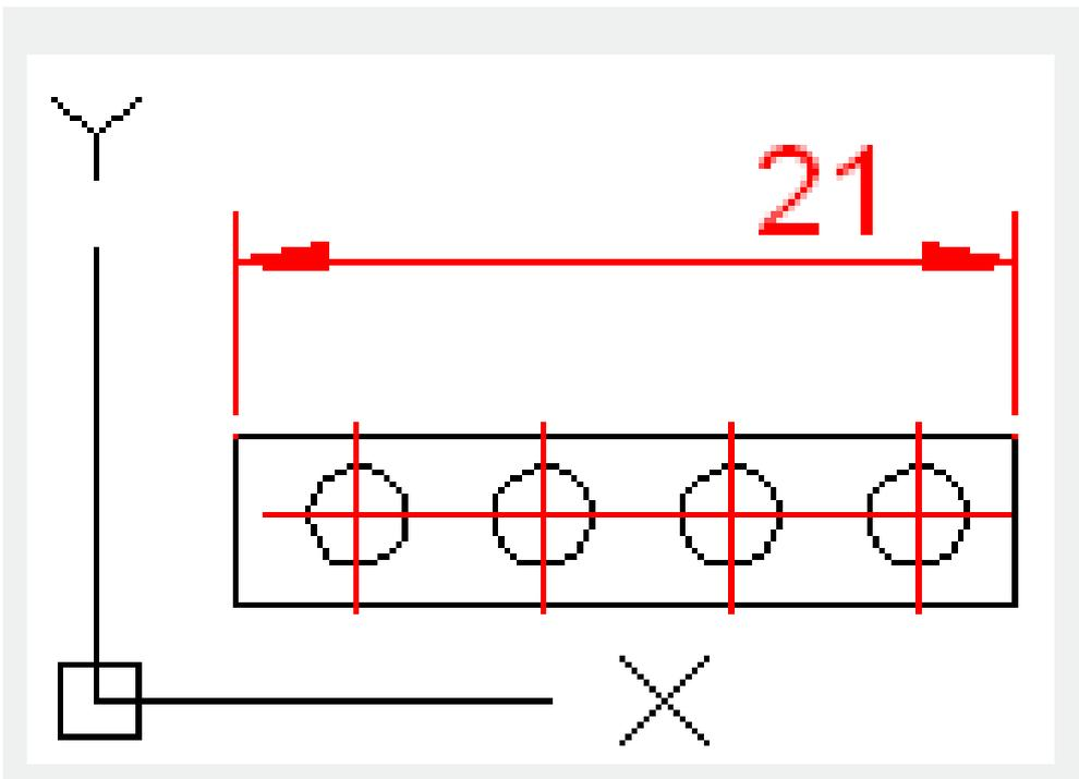
**Center** : The dimension text is in the middle of dimension line, this option is only applicable to linear, radius and diameter dimension.
