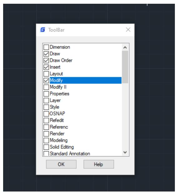
A toolbar can be displayed as floating or docked. A floating toolbar will show anywhere in the drawing area and it can be dragged to a new location, resized, or docked. To dock a toolbar, you can attach it to any edge of the drawing area. If you dock the toolbar at the top edge of the drawing area, it will show below the ribbon. To move a docked toolbar, you just have to drag it to a new docking location.
