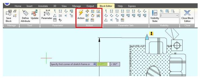
**Move**: Move action causes objects to move a specified distance and angle such as a point, a linear, a polar, an XY parameter, etc, moves all objects in a selection set in a/any direction.
