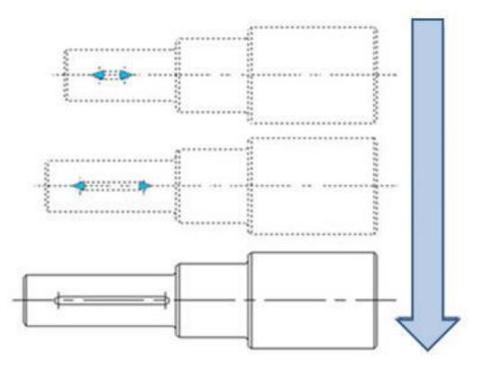
The realization of chain action has two important procedures: First, modify the property value of the parameter that needs to happen linkage and modify the property of "chain action" from "NO" to "YES". Second, select the parameter of objects that selected to linkage action to set.
