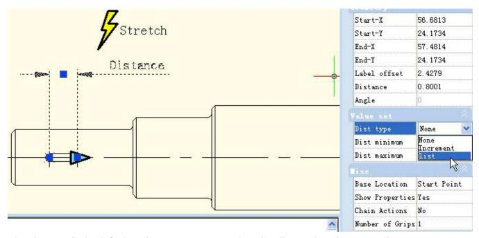
Therein, none is the default option, means can stretch optionally. By the other two options, you can define the maximum and minimum numbers respectively.
