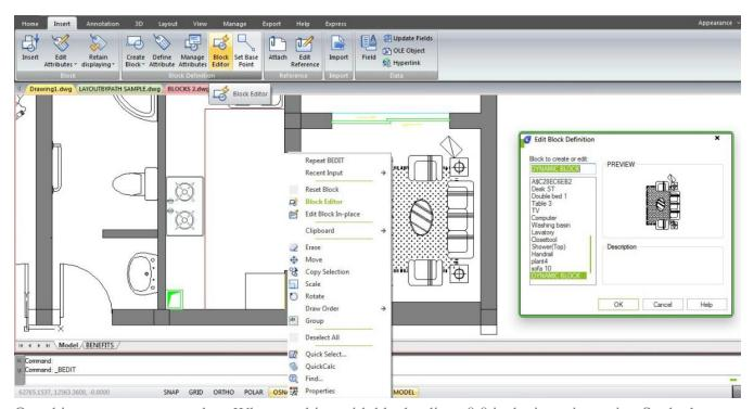
One thing you must remember. When working with block editor, 0,0 is the insertion point. So don't move the geometry unless you want to move the insertion point!
