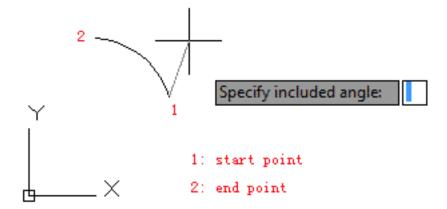
• **Direction**: Create an arc from start point to endpoint and specify the tangent line direction of the start point. Users only need to determine tangency direction without regard to anticlockwise or clockwise, major arc or minor arc.
