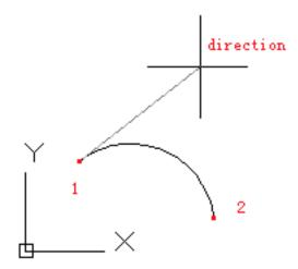
• Radius : Create a minor arc from the start point to end point. If inputting a negative value for radius, it will create a major arc.
