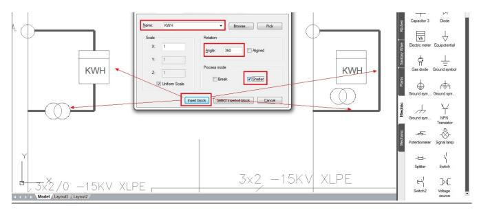
Technical Demo - Block Break is another innovative tool. It allows you to wipeout or break an object that is overlapped by a block definition.
