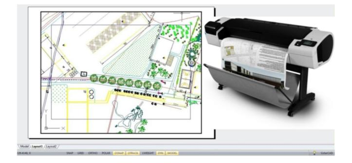
Instead of manually configuring the PLOT command for each drawing, you can use Named Page Setups to change the same settings for your drawing layout 1, 2, 3, and so on.
