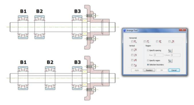
Another example, we can apply this tool for arrange the part numbers distribution over the leader lines. Notice that the objects to be selected are Mtext and will be distributed according to the top object level as a reference. After started the command, a prompt message will display > Please select the object to arrange:
