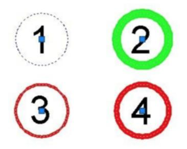
Only block no.2 using the block properties, because we set it the geometry properties to by block. Now freeze Layer1. We can see the block no. 4 disappeared, because the object in it was created on it.
