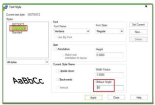
Now try to create text (single or multi line) with different styles and angle combination, then change the rotation to 30 deg or -30 deg. It depends on where you want to put it. See next image as reference.
