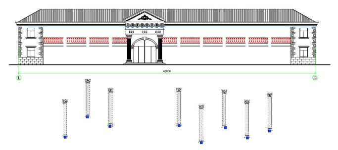
Please note that the columns are not aligned at same position to each other and they are independent blocks. In this case, we will perform Top object Y axis and specified object alignment.
