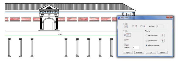
After the objects have been aligned, we have to select the option specified object under Align to. Then select the object (blue line) where we want to align and place the objects. Finally you will get a faster result performing this operation:
